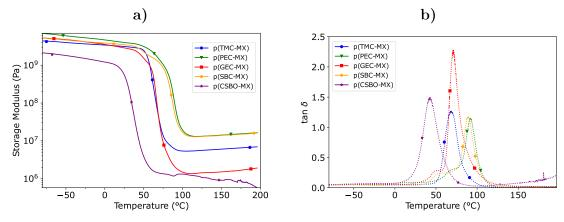
Figure 4. Dynamical mechanical analysis of the PHU thermosets. (a) Storage modulus evolution with temperature and (b)  $\tan \delta$  evolution.
