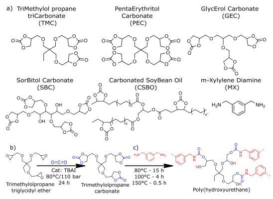
Figure 1. (a) Idealized (macro)molecular structures of the resins precursors and (b) model reaction from TMPTGE epoxy monomer to TMC cyclic carbonate to (c) p(TMC-MX) PHU thermoset.
