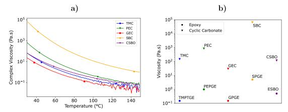
Figure 2. (a)Viscosity evolution of the cyclic carbonates over temperature and (b) comparison of the viscosity of epoxy and carbonate monomers at 25 °C.
