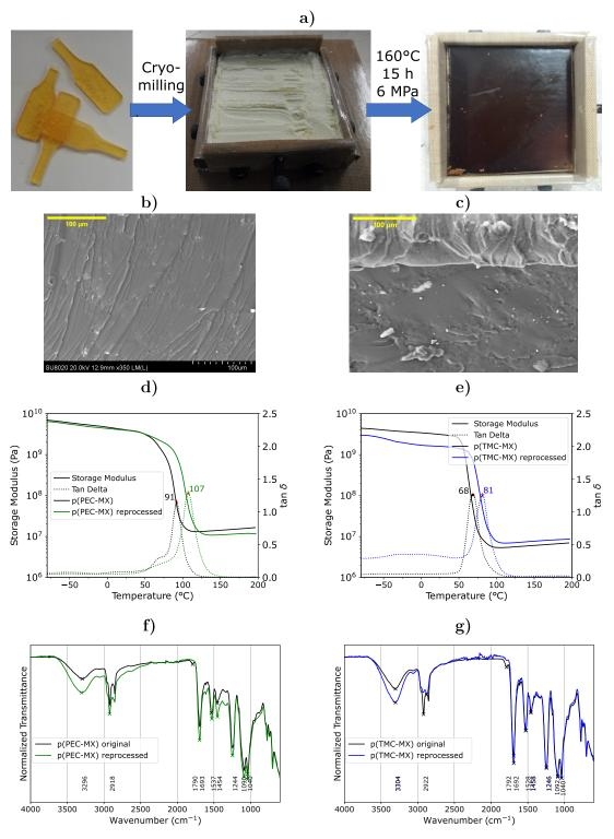
Figure 7. Reprocessing of PHUs. (a) General protocol and reprocessed p(PEC-MX), (b, c) SEM picture of freeze-fractured p(PEC-MX) and p(TMC-MX), (d, e) DMA of p(PEC-MX)and p(TMC-MX), and (f, g) FTIR of p(PEC-MX)and p(TMC-MX).
