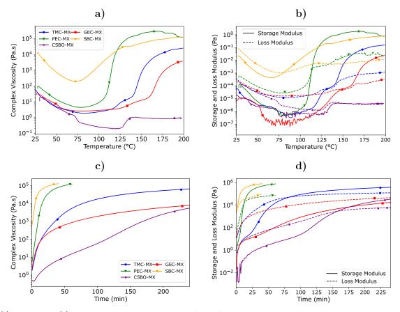
Figure 3. (a) Viscosity and (b) storage and loss modulus evolution of PHU formulations during nonisothermal curing rheological analyses. (c) Viscosity and (d) storage and loss modulus evolution of PHU formulations during isothermal curing.
